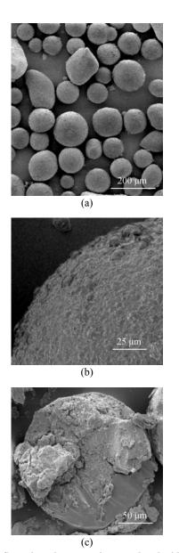
Figure 1 Scanning electron micrographs elucidating the microstructure of the toxin-loaded formulation: (a) general external appearance of the particles; (b) detail of a particle's external surface; (c) inside of a fractured particle
