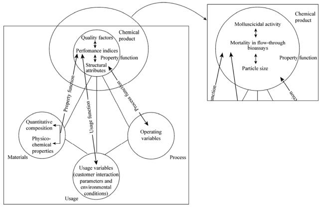
Figure 3 Completing a chemical product pyramid for particulate poisons
