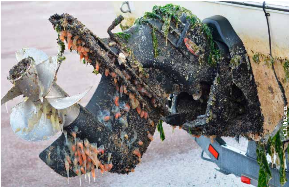
Figure 1. Biofouling on the motor of a pleasure boat.
