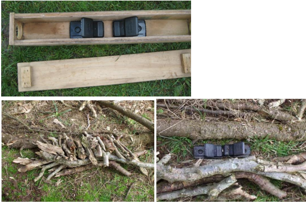
Figure A2.1 - Above: Two (set) Trapper T-Rex™ traps back to back in a homemade wooden tunnel. The entrance to the tunnel restricts entry by larger species and prevents the trap being dragged away. The gap between traps prevents them setting each other off. Below: The same in a natural tunnel made of branches (shown both open and covered). Images © WMIL.
