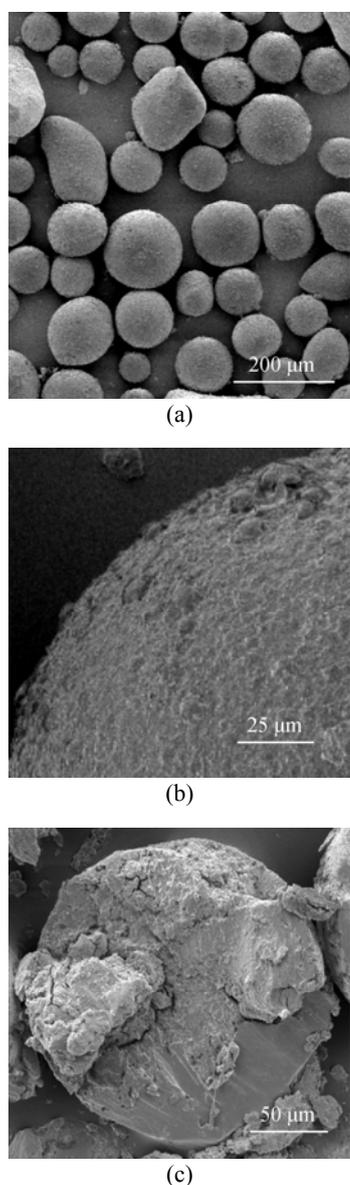
**Figure 1** Scanning electron micrographs elucidating the microstructure of the toxin-loaded formulation: (a) general external appearance of the particles; (b) detail of a particle's external surface; (c) inside of a fractured particle
