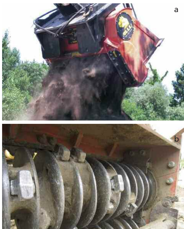
Mechanised management of knotweed in the Gard department, a) soil grinding, b) grinding rotor in the bucket.
