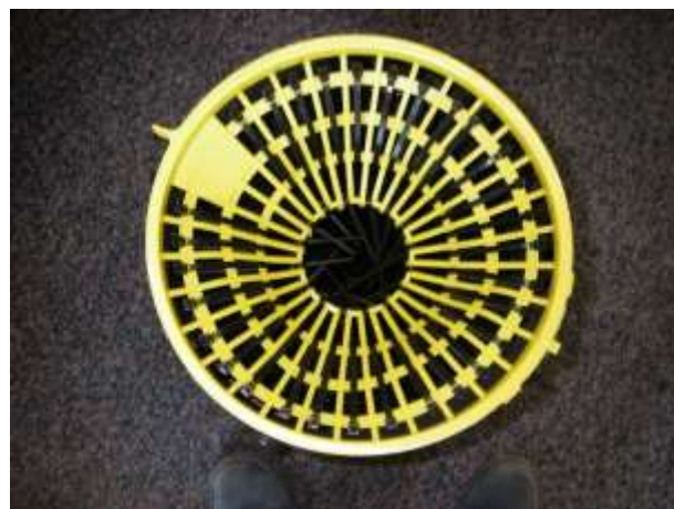
Figure 9. Increased trap entrance diameter, also zip ties added to limit mesh size on the funnels, zip ties can also be observed internal to the trap.
