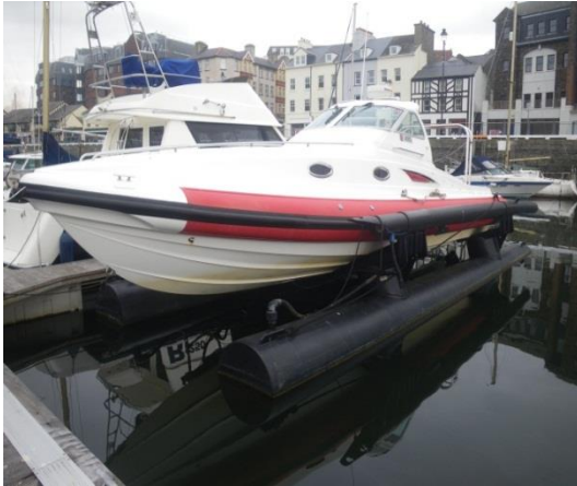
Floatation system used to store vessels out of the water whilst not in use. Photo © E. Cook, SAMS
