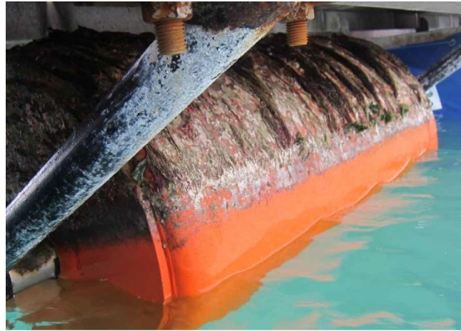
Rotating pontoon floats under trial in North Wales. Photo © Rohan Holt. NRW
