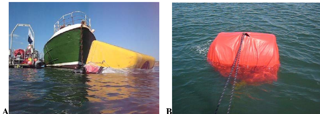
Figure 26 Wrapping large mooring buoys. A, Largest of the mooring buoys treated; B, Medium-sized buoy wrapped using two adapted finger pontoon bags.
