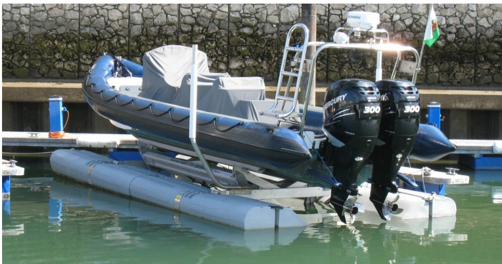
Figure 46 Photo: R. Holt. Sunstream boat lift supporting an rigid hulled inflatable at Deganwy marina, Conwy.
