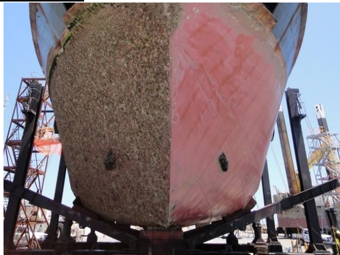
50:50 cleaned hull Image courtesy of Envirocart https://www.grdfranmarine.com.au/
