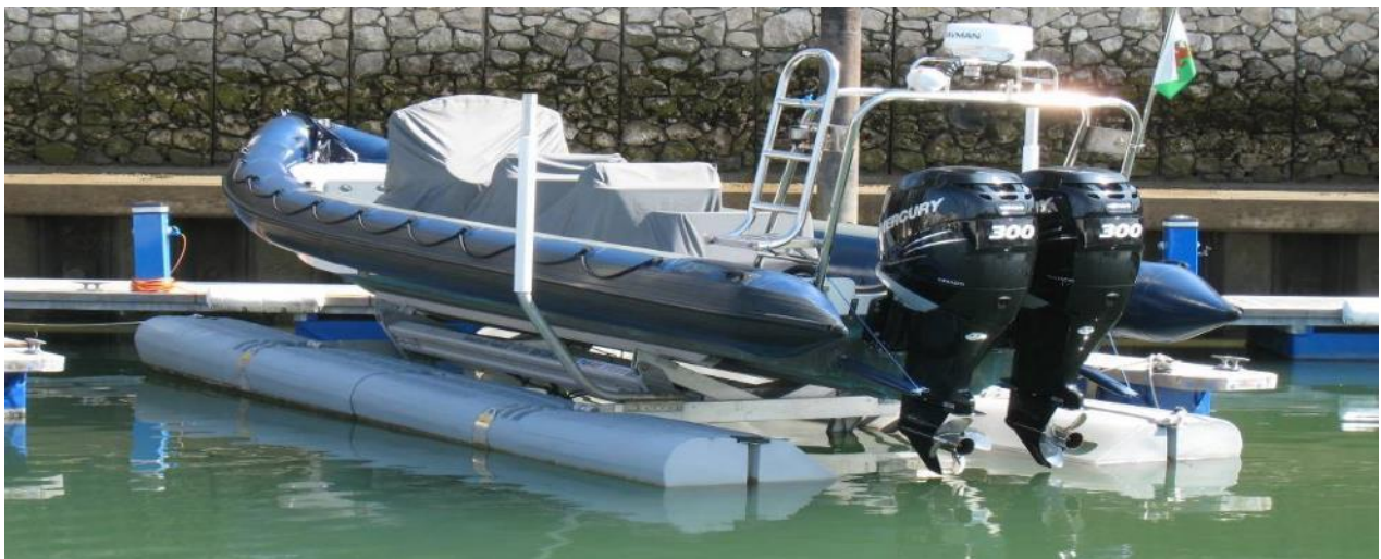
Sunstream boat lift supporting a rigid hulled inflatable at Deganwy marina, Conwy. Image courtesy of Rohan Holt, Natural Resources Wales
